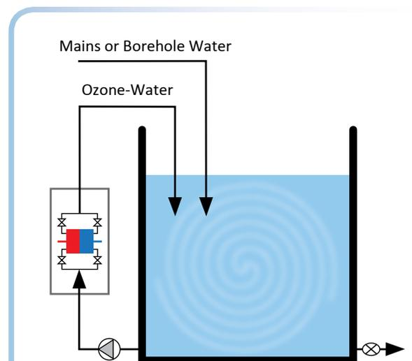
In this tank circulation system, water is simply drawn from the bottom of the tank, passes through the **DiaZone**<sup>®</sup> cell and returns to the top of the tank. The ozonated water generated by the cell rapidly diffuses through the body of the water in the tank. Ozone in solution rapidly disinfects water and also sanitises the internal surfaces of the tank, below and above the water line. Tanks treated this way are maintained in a sparkling clean condition!
